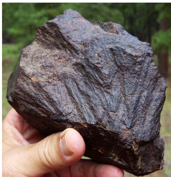
Figure 1. Shatter-coned 1.74 kg NWA chondrite.
